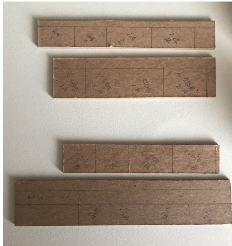
Binders board that is measured and ready to be cut.
