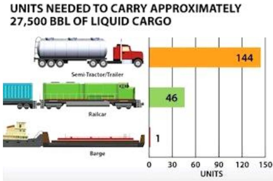
Figure 2, Barge to truck and rail car liquid comparison.
