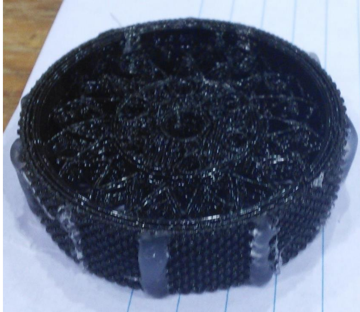
Figure 3. Angled view of attempted spiked wheel. Hot glue was placed to try to increase traction, but ultimately decreased it.
