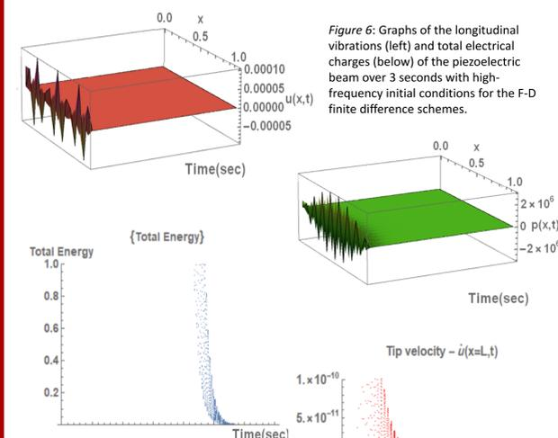
Figure 6: Graphs of the longitudinal vibrations (left) and total electrical charges (below) of the piezoelectric beam over 3 seconds with high-frequency initial conditions for the F-D finite difference schemes.
