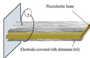
Figure 1: A piezoelectric beam covered with aluminum foil, clamped at one end and free at the other.
