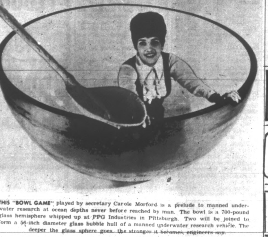
THIS "BOWL GAME" played by secretary Carole Morford is a prelude to manned underwater research at ocean depths never before reached by man. The bowl is a 700-pound glass hemisphere whipped up at PPG Industries in Pittsburgh. Two will be joined to form a 56-inch diameter glass bubble hull of a manned underwater research vehicle. The deeper the glass sphere goes, the stronger it becomes, engineers say.
